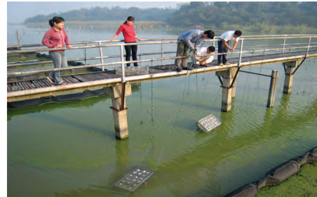
The researchers lowered the bioassay containers into Lake Taihu in frames and left them to incubate under natural light and temperature conditions for up to 4 days. Each day they measured the algal growth response. © Hans Paerl/University of North Carolina at Chapel Hill
