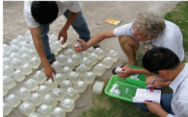
In 2013 Hans Paerl and Chinese colleagues conducted bioassays at Lake Taihu to assess the impact of nutrient enrichment on cyanobacterial blooms. The containers were filled with lake water treated with various concentrations of nitrogen and phosphorus to show how the nutrients affected the lake's natural algal community. Hans Paerl/University of North Carolina at Chapel Hill
